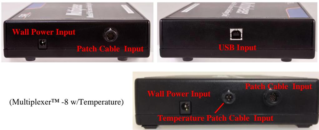
To set up the system, connect the Patch Cable into the mating port on the Multiplexer™, then connect the other end of the Patch Cable into the **Universal Cable Input** on the MouseOx® Plus. The two systems can be stacked to reduce their overall footprint on the lab bench. The Multiplexer™ - 8 w/Temperature has an
