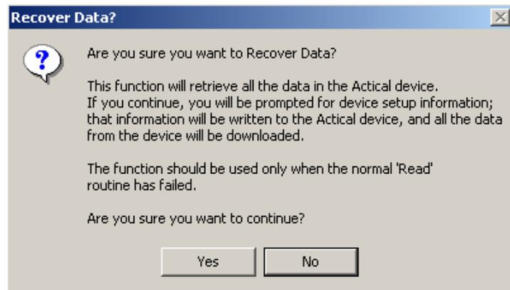
The recovery header generates a new header based on input from the following prompt.
