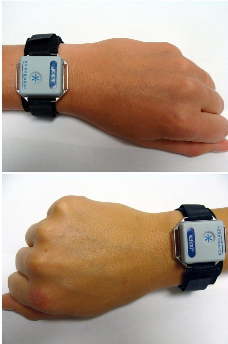
When placed on the band correctly, the Respiration logo will be parallel to the band and on the edge of the device nearest the elbow.
